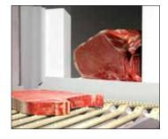
Dynamic portion separation ensures that even bone-in or frozen and solid products are deposited cleanly. At the precise moment the slice is cut, it moves upward briefly. Thanks to this precise separation, the slices are prepared optimally for further processing like e.g. packaging.
