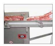
Loading takes place continuously via a conveyor belt. Products are automatically transported to the cutting area.
