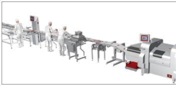
The Smartline (above) is an automatic solution. A spice/marinating station can optimally be integrated. The latest robot technology supports fully automatic sorting and infeeding (below).
