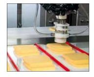
The FALCON hybrid+ is of course also ideal for processing cheese. The robotic version boasts the latest robot technology for fully automatic sorting and infeeding. Up to 100 picks per minute are possible.
