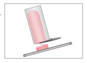
Static Distance Control (SDC): The placement table is positioned before the slicing process for optimum placement of the slices.
