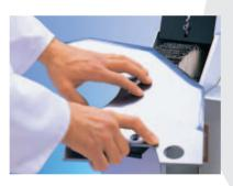
**Polishing and deburring:** The cutting edge manually is given its final fine trim on the finned brush. Exactly appropriate peripheral speed and optimally adjusted brush resistance protect the cutting edge and level out handling errors.
