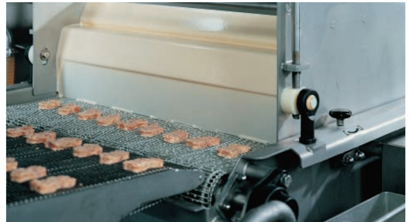
Batter curtains apply batter to the top and sides of the product.
