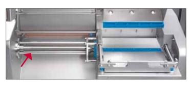
Thanks to the open design, everything is easily accessible, even the hydraulic feed cylinder (see arrow). The feed cylinder with which the CASAN 200 is equipped as standard is also called the hygiene cylinder because it makes product contamination with hydraulic oil (only foodstuff hydraulic oil is employed at TREIF) technically impossible. No oil can get into the cutting chamber.
