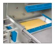
The cheese is fed automatically with just the hydraulic pressure necessary for a good cutting result with the set parameters. That is gentle on the product and energy as well as hydraulic oil can be saved compared with conventional systems.
