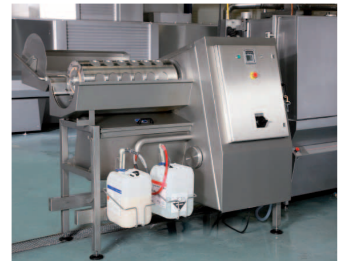
The cleaning unit cleans portioning drums fully automatically both inside and outside
