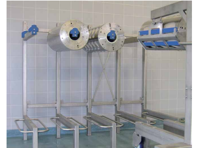
The lifting unit easily moves the portioning drums to the cleaning unit or to the storage rack
