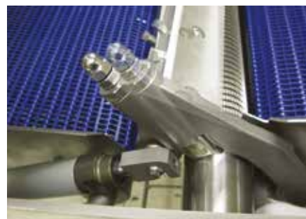
Open-bite adjustment, which ensures a positive skinning start, is built into the open-bit cylinders and spring cartridges
