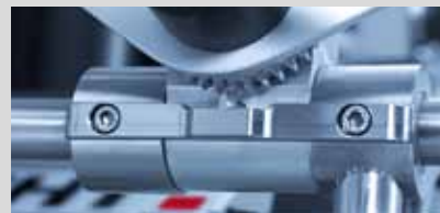
Locking mechanism used to change knives
