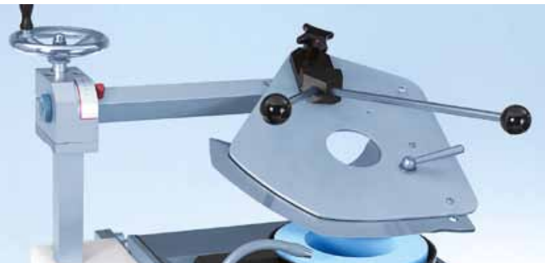
Standard grinding arm for sickle-shaped bowl cutter knives
