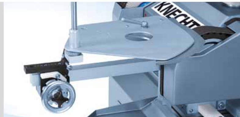
Belt grinding attachment HV 261 for sickle-shaped bowl cutter knives
