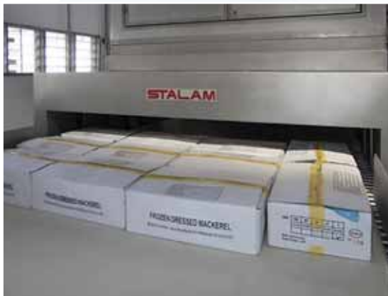
"RF 85 kW" defrosting equipment for mackerels.
