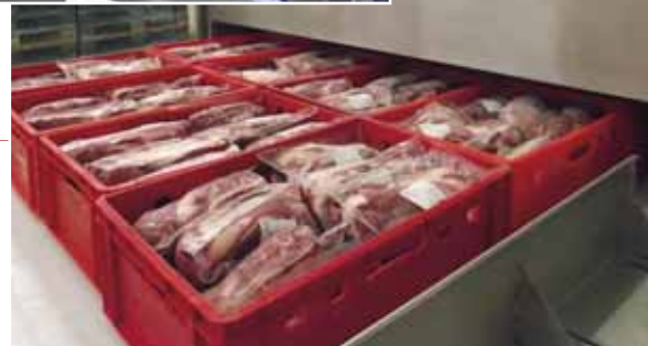
"RF 4x60 kW" defrosting equipment for pork and beef.
