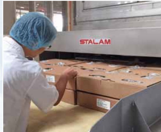
"RF 85 kW" defrosting equipment for herrings, hallibuts, grey sole.
