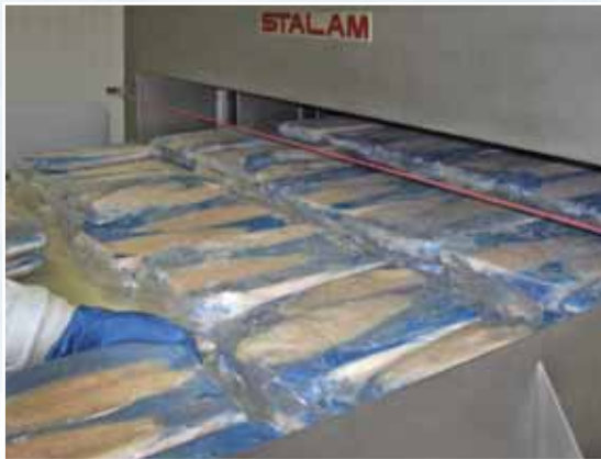
"RF 85 kW" defrosting equipment for fish fillets.
