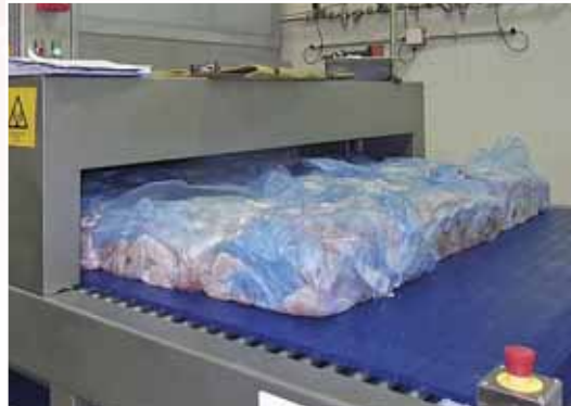
"RF 85 kW" defrosting equipment for pork.
