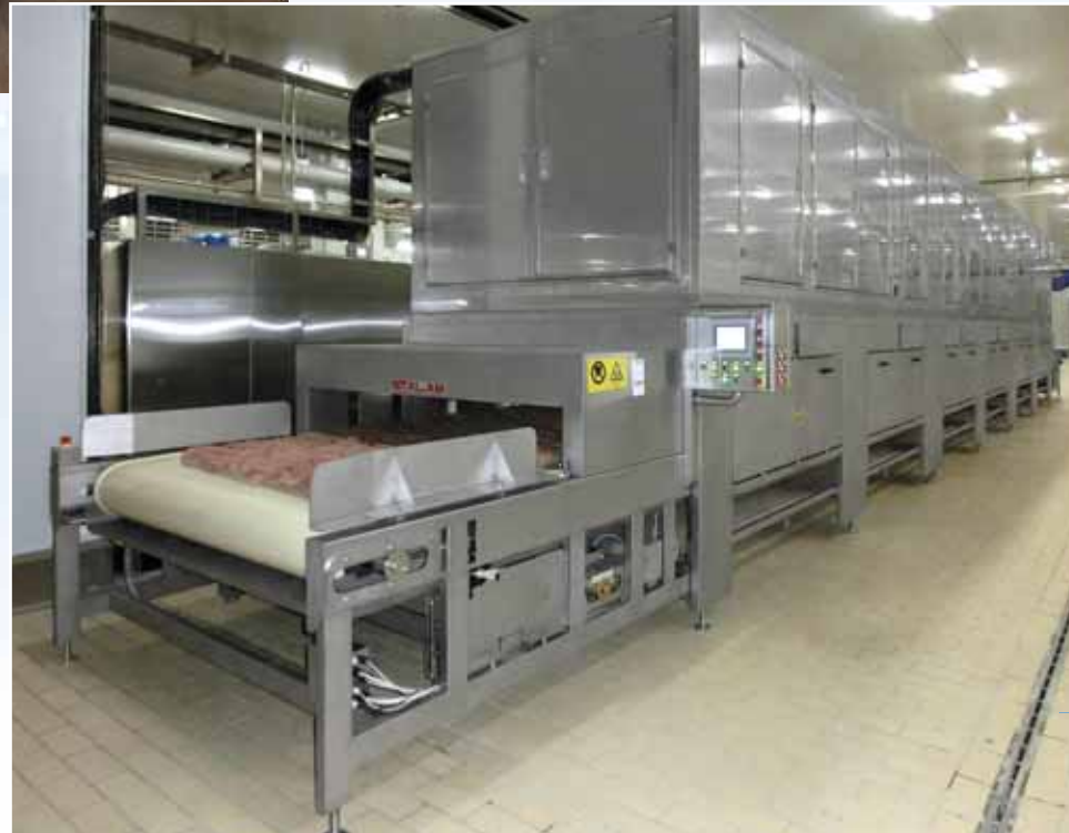
"RF 85 kW" defrosting equipment for mackerels and sardines.
