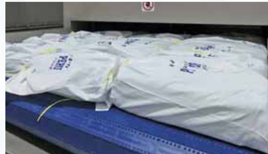
"RF 85 kW" defrosting equipment for squid, shrimps, etc.
