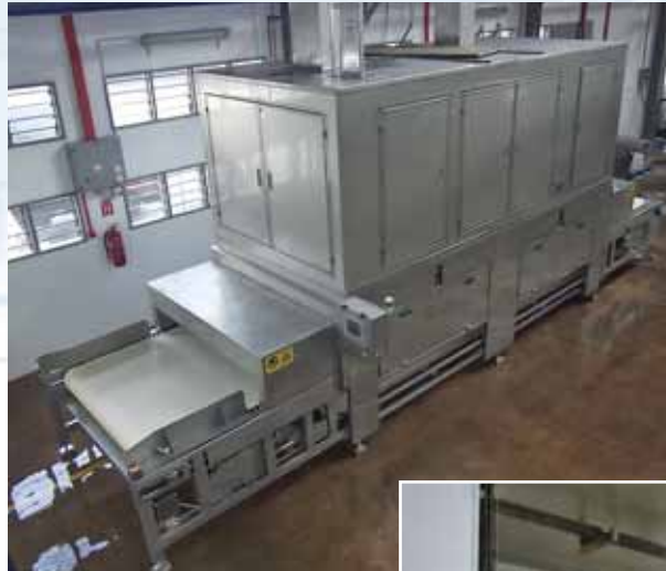
"RF 85 kW" defrosting equipment for mackerels and sardines.
