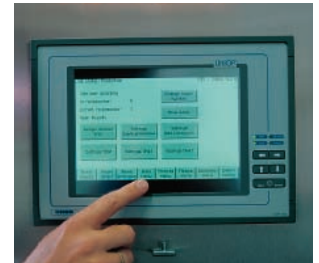
Operation of the oven is by means of a menu on a touch screen.
