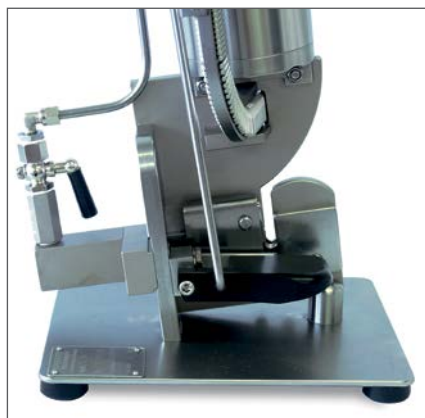
Triggering of the sensing lever and cutting knife that can be shut off.
