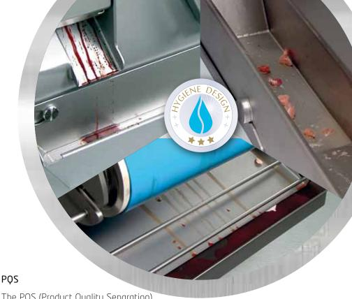
The PQS (Product Quality Separation) prevents possible product residues from entering the OK material. The gridset is shielded by the PQS (also see photo above) so that residual material drops behind the wall where it is collected.
